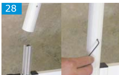
WHERE VERTICAL SUPPORT POLE IS PRESENT: With the curtain rail in position, guide the post extension over the post spigot and secure in position with the supplied grub screw. Depending on your enclosure type you will secure the post to the curtain rail or using a boomerang bracket.
