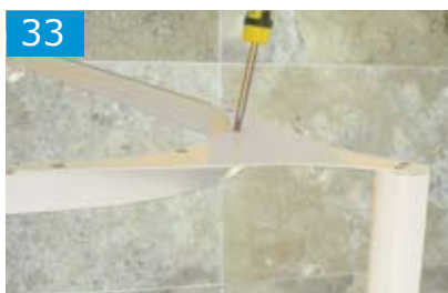
Screw the boomerang bracket to the curtain rail using the No6 x 3/4" countersunk screws. USE SCREWS PROVIDED.
