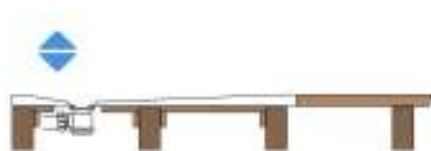
Tray can be easily recessed into a wooden floor
