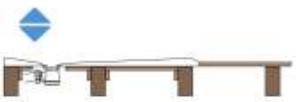
The tray can be recessed into a wooden floor
