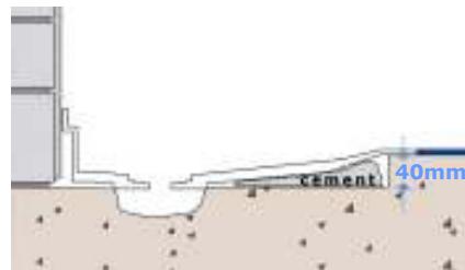
Void under the tray filled with a weak sand and cement mix
